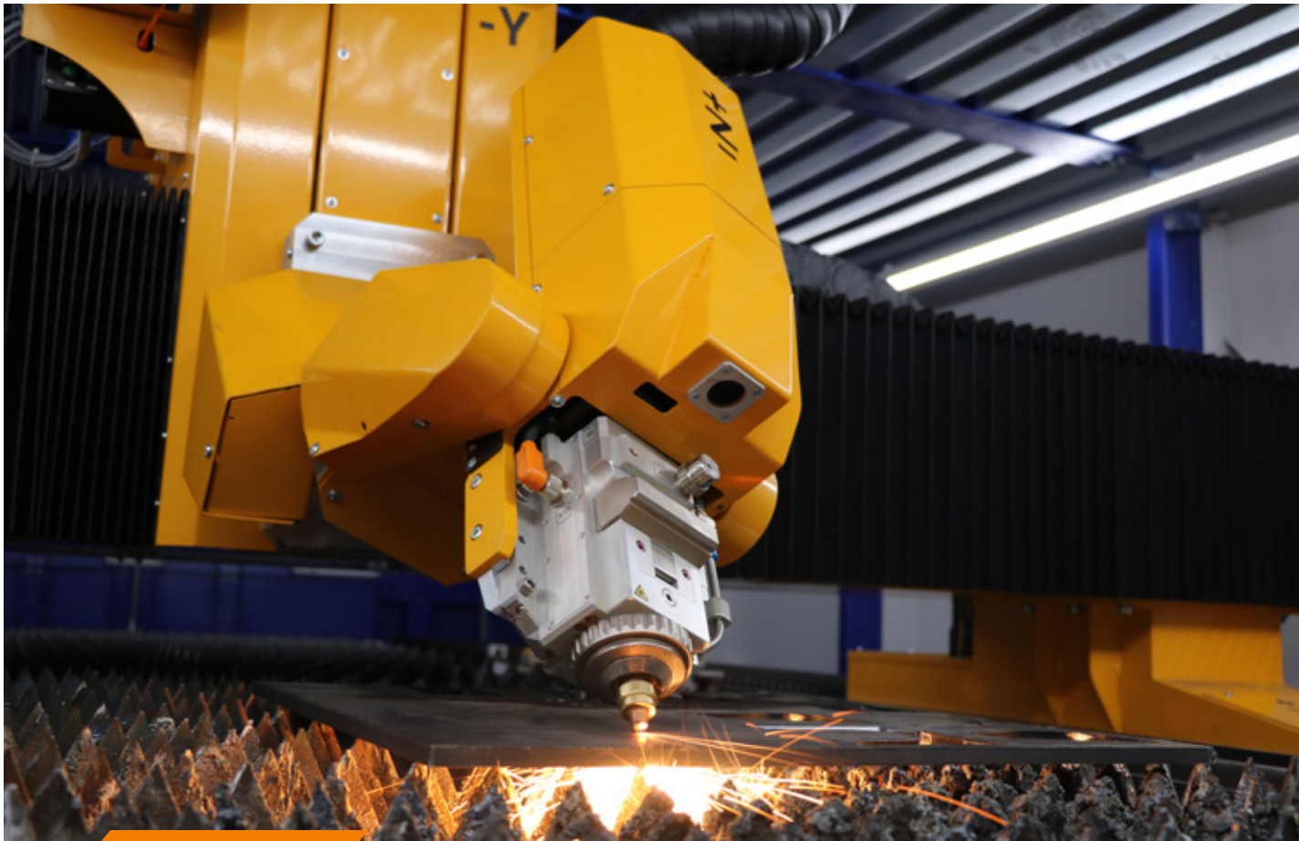
↑ In addition to its plasma offerings, fiber laser bevel cutting up to 45 degrees is also available from United Precision.
