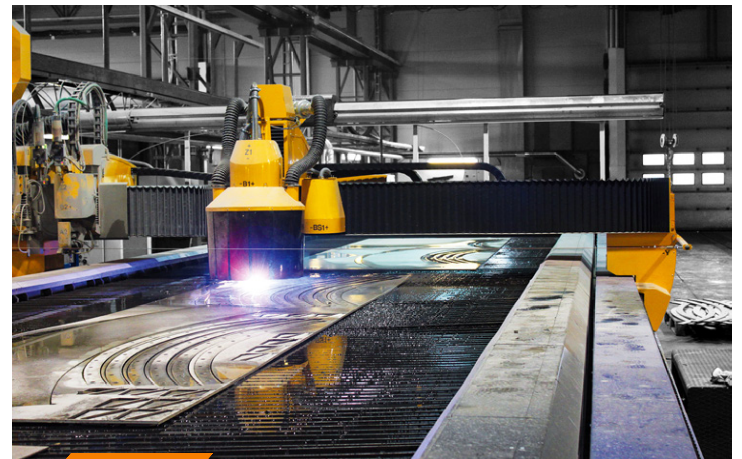
↑ Plasma and waterjet technologies can be combined on a single cutting plan, as shown here.
