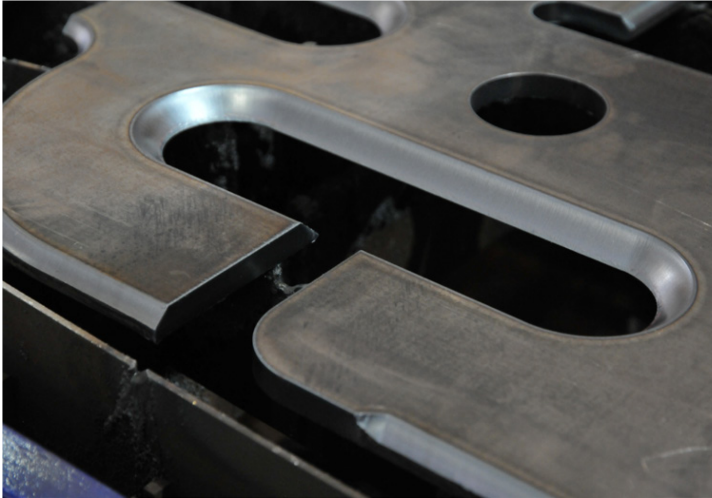
The MicroStep Rotator cutting head's degree of bevel varies for each technology it's paired with. For fiber laser and waterjet, 45-degree bevels are possible. For plasma, it's 50 degrees. For oxyfuel, it's 65 degrees.
