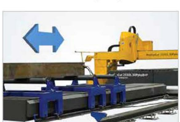
Thanks to the large, open loading area, even heavy beams can be easily and safely slid over the supporting rollers into the work zone. This saves time as the beams do not have to be clamped or otherwise prepared for processing.
