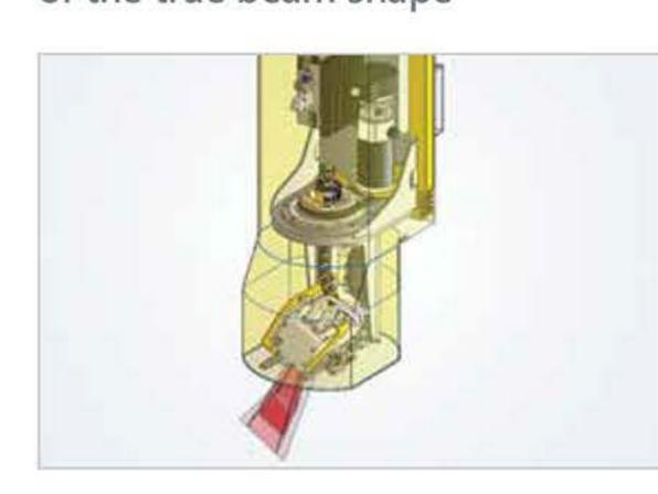
ProfileCut machines are equipped with a 3D laser scanner that measures the exact shape of beam in the place of cutting. Advanced algorithms then allow the control system to adjust the movement of tool accordingly and compensate for possible inaccuracies of the particular beam.
