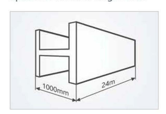
Thanks to its generous work areas, the machine can process beams up to HEB 1000 and a length of 24,000 mm. In addition to the common beam types such as I, H, U or L, round pipes, hollow sections and even domes and plates can be cut as well.
