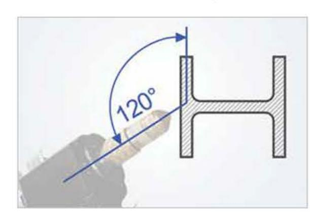
MicroStep's 3D rotator with a torch tilt of up to 120° provides full beam processing functionality including dividing of beams and cutting of commonly required contours and openings. The advanced auto-calibration feature (ACTG®) guarantees long-term accuracy, easy setup and minimum maintenance downtimes of the bevel cutting equipment.
