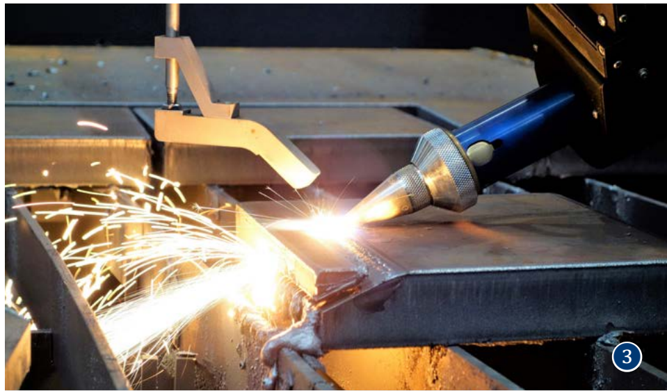
Oxyfuel bevel cutting of sheet metal - preparation of „top Y“ shaped weld surface
