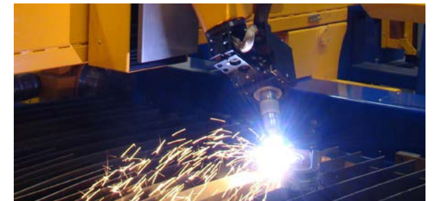
With beveling technology from MicroStep, V-, Y-, and (under certain conditions) also X- and K-cuts can be added to already pre-cut parts.
