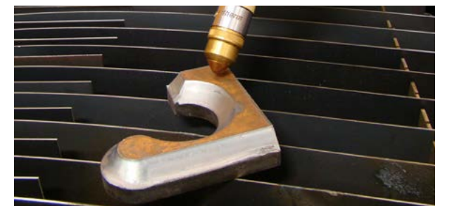
Thanks to high rigidity of the cutting machine, the cutting results are finer and more precise than with a robot.
