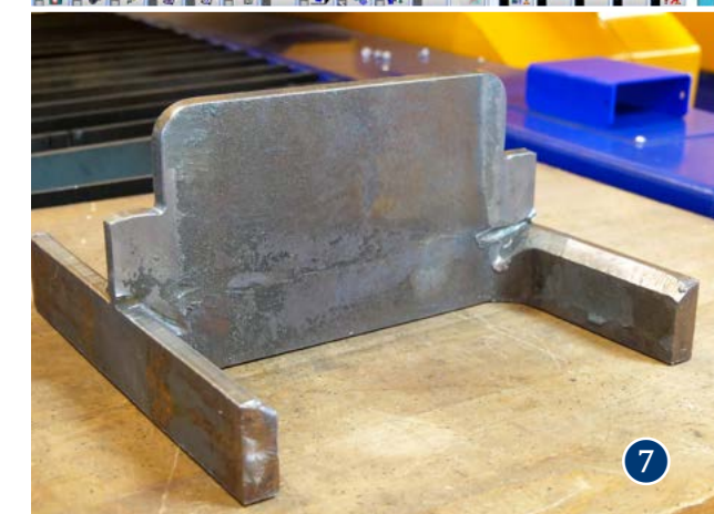
Top: Screenshot from the MicroStep mSCNC control system with loaded cutting program for cutting the web of H beam (output from the 3D CAM software mCAM); Bottom: Final cut part.
