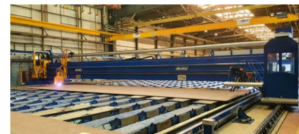
In 2020, the shipyard invested in two panel processing lines which include two 20.5 m wide MicroStep gantries for bevel cutting, primer removal and marking of large-scale panels.
