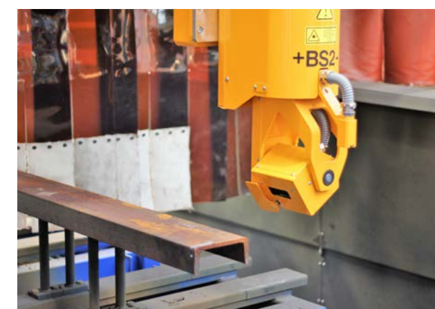
Plasma pipe cutting. The large positioner enables cutting of pipes up to Ø 2,000 mm, length 6 m and weight 7 tons.
