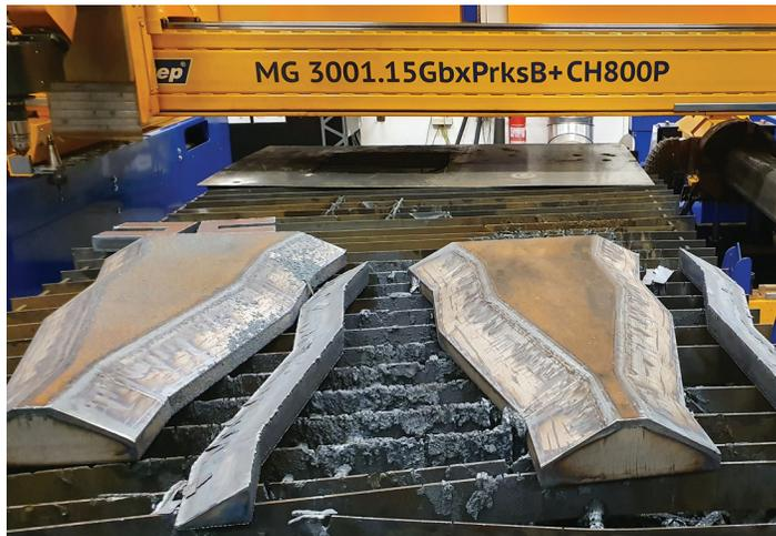
Advantages of additional beveling with oxyfuel: minimum waste, smooth cut surfaces, precise cut contours also for bigger bevel angles, as showcased on the above parts 3.55" thick, Y cut with land size 0.8", bevel angle 60°, cut with MicroStep ABP technology for a South African customer.
