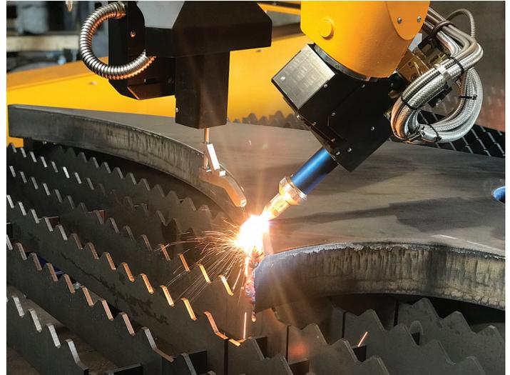
Oxyfuel rotator for weld preparation on thick metals utilizes MicroStep's patented ACTG technology for automatic compensation of kinematic inaccuracies, and thus delivers reliable cutting results in the long run with less frequent maintenance necessary.
