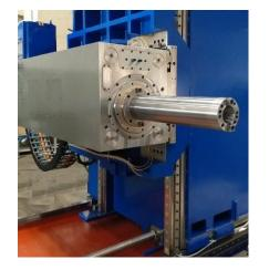
The spindle Ø 5.1 in, located inside the RAM, is made of forged and tempered alloy steel and assembled with high precision ball bearings.
