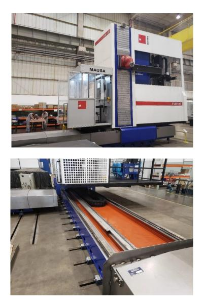
The longitudinal movement of the column, X axis, is transmitted through two sets of servo motors and planetary reducers of high precision, in the "master / slave" configuration, producing uniform and smooth movements, eliminating "backlash" in the reversals movement.
