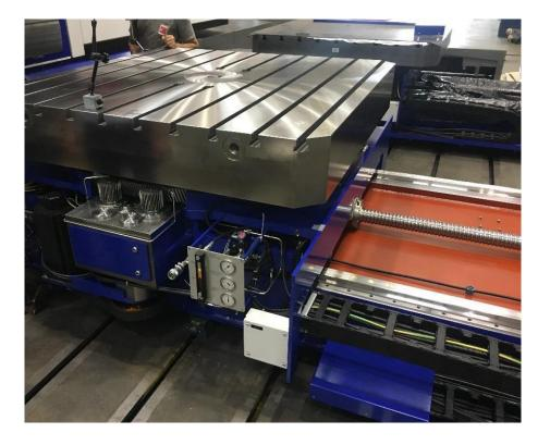
The rotational movement of the table of 33,069 or 66,139 lbs, axis B, on the base, is supported by a hydrostatic system, which consists of a pressurized oil film permanently between the surfaces, eliminating the contact, as well as the consequent wear between the parts . Transmission is performed by a servomotor and two preloaded pinions, eliminating backlash clearance issues
