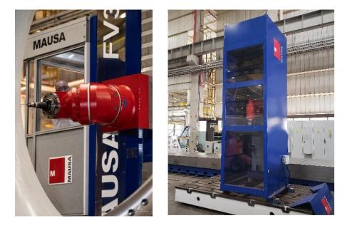
It can be configured with Milling Heads of different models and "pick-up" station for automatic head changing.
