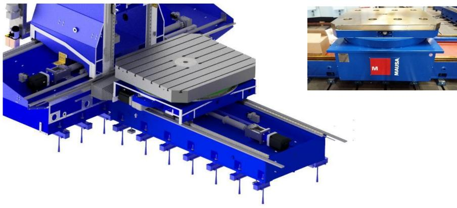
The rotational movement of the table, axis B, on the base, is supported by a hydrostatic system, which consists of a pressurized oil film permanently between the surfaces, eliminating the contact, as well as the consequent wear between the parts.
