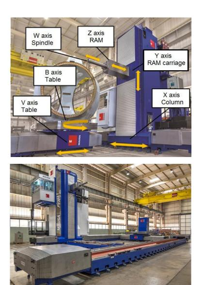
The CNC Boring Machine FV 301 has robust structure and design concepts, to meet a wide range of medium and large parts applications, which require high chip removal rates, combined with a high degree of precision.
