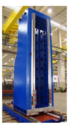
The headstock is positioned in the center of the doublewalled column, in the "Box in Box" concept, having two front and rear guides, providing great geometric stability and high rigidity, responding uniformly to machining forces, regardless of cutting directions.
