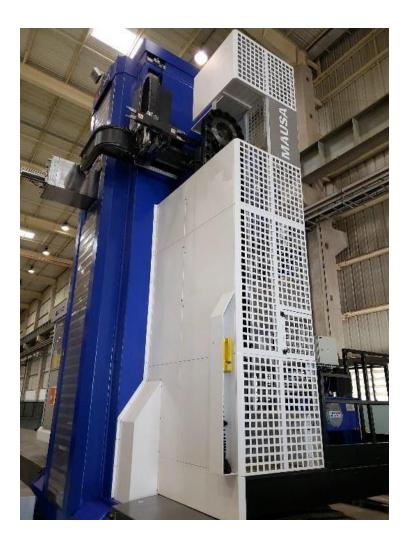
The CNC Boring Machine FV 301 is equipped with an Automatic Tool Changer, with a magazine for 60 or 120 positions.
