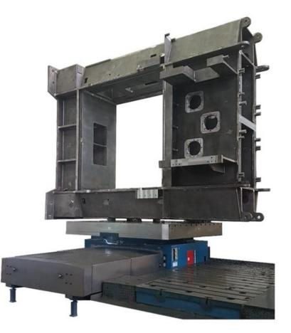
The rotational movement of the table of 66,139 / 132,277 / 220,462 lbs, B axis, on the base, is supported by a hydrostatic system, which consists of a pressurized oil film permanently between the surfaces, eliminating the contact, as well as the consequent wear between the parts.
