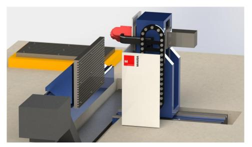
This arrangement provides excellent distribution of forces and stability during machining efforts. The table surface is 90 degrees from the ground and its movement in the direction of the X axis is transmitted through a ball screw and brushless servomotor. It has direct measurement on all axes, using optical
