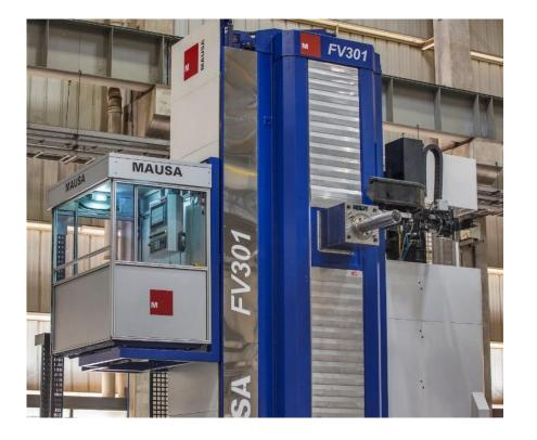
The vertical movement (Y axis) of the RAM car, in the column, is performed by two servomotors, in gantry arrangement and transmitted through two Ø80mm ball screws, positioned symmetrically in the front part of the column.
