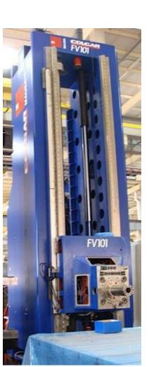
The lubrication is achieved by means of a special system, air-oil, lubricating and cooling the entire assembly, allowing uninterrupted work at high rpm
