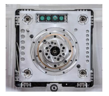
The spindle Ø 6.3 in, located inside the RAM, is made of forged and tempered alloy steel and assembled with high precision ball bearings
