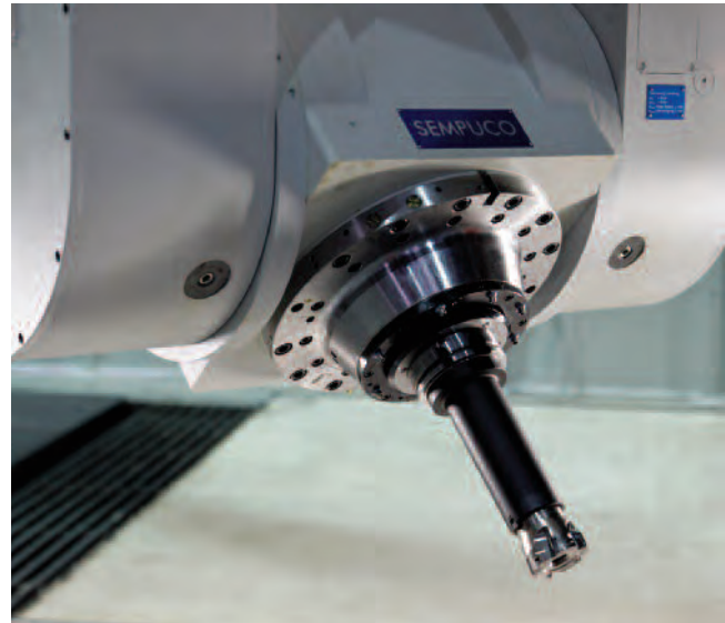
2-axis swivel head with 9,000 rpm
