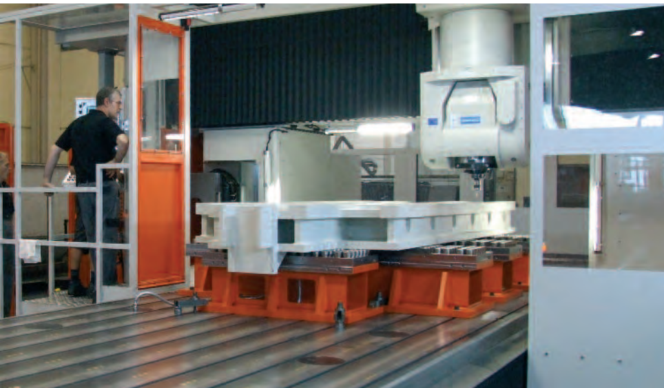
matec-40 P with 2-axis swivel head
