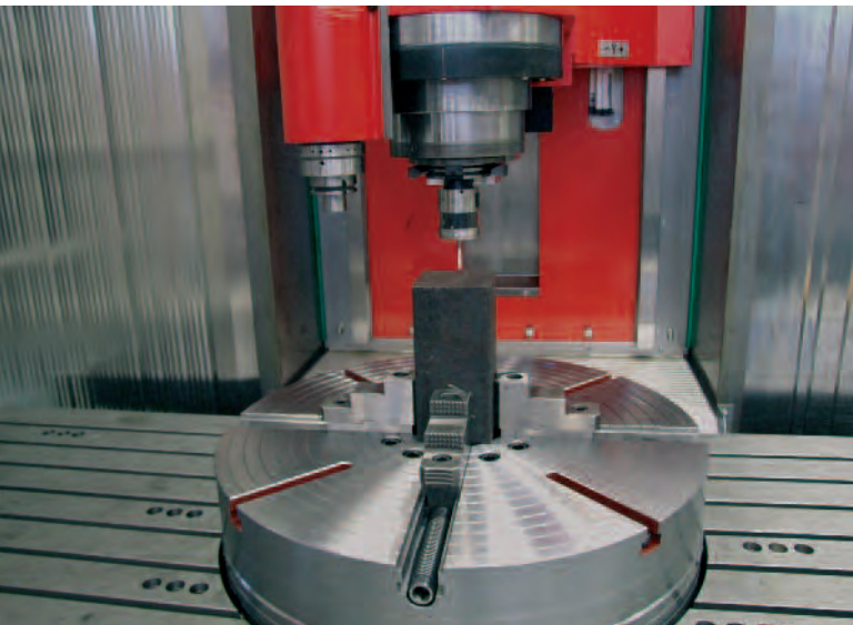
Working area with integrated rotary table and mounted jaw chuck
