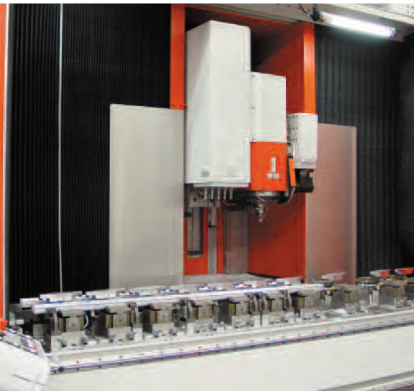
matec-30 L special clamping devices for aluminium profiles
