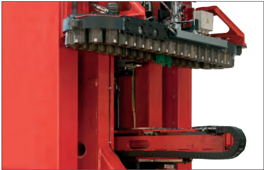
Tool magazine HSK-A 100 for 40 or 60 tools
