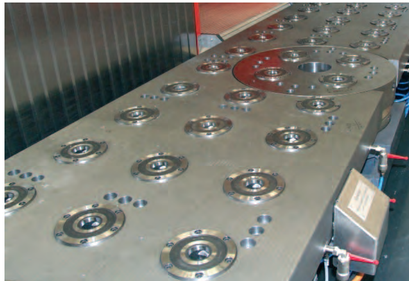
Machine table with integrated rotary table and mounted quick change pallet system
