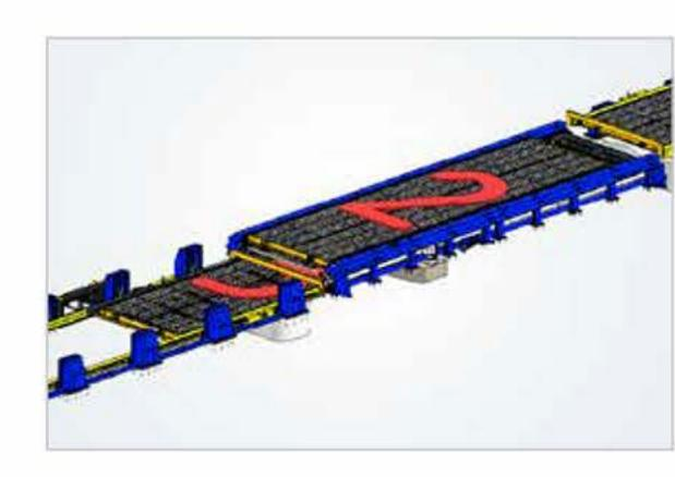
The system consists of 3 separate working zones that allow simultaneous operations of loading/unloading and work-piece machining, e.g. cutting, marking, primer removal... Table exchange between zones is synchronized to enable highest possible efficiency of production.
