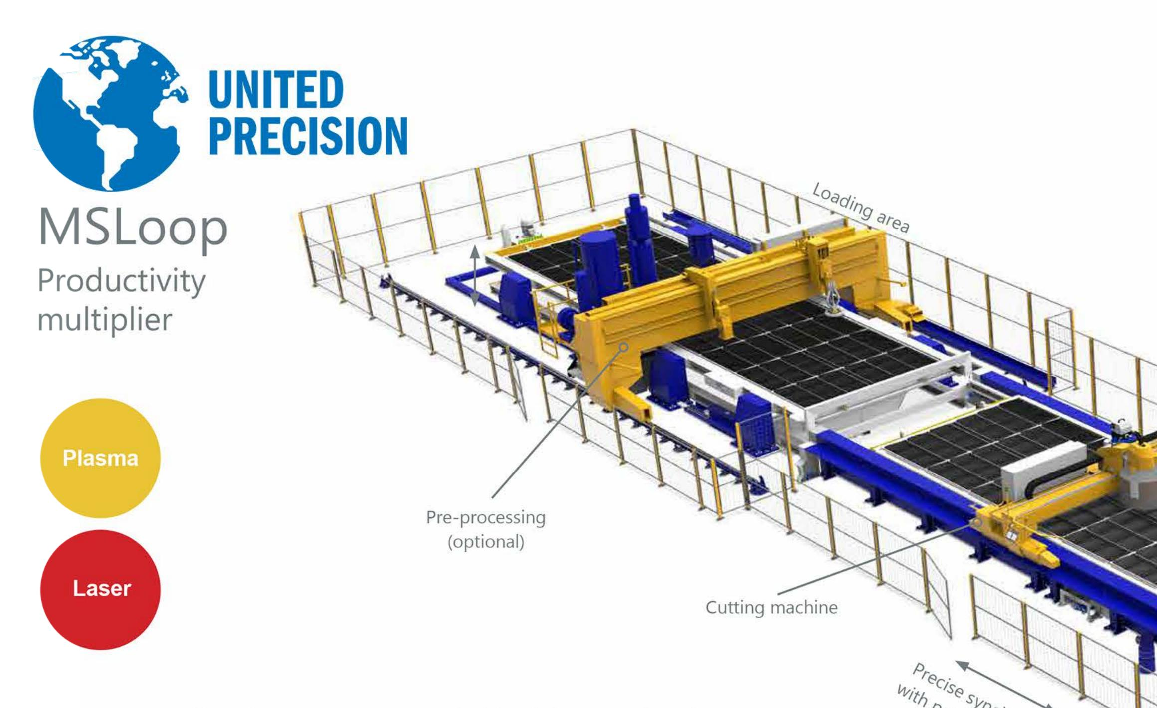
The automated table exchange system **MSLoop** significantly increases throughput of a CNC cutting machine as it allows simultaneous loading, cutting and unloading of material. Its three grates exchange in a continuous loop, with the returning grate moving underneath the CNC machine. The grate size of MSLoop is customizable in 1.5 m length modules.
