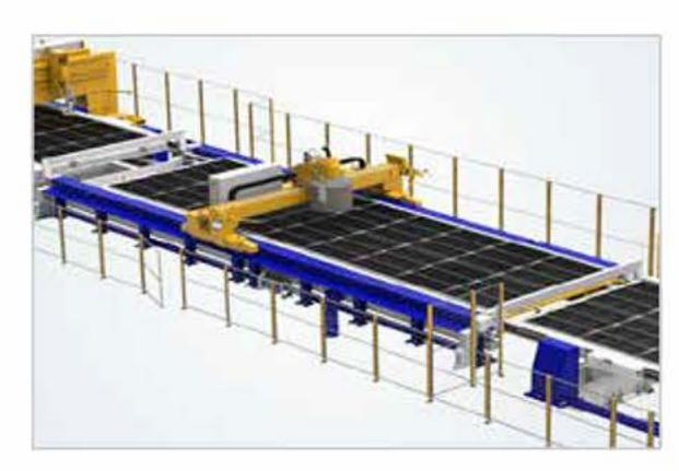
Each zone has its own entrance into the fenced-off area that unlocks from the outside only after all the machinery in the zone finishes its movement and is switched to a manual slow-moving mode. The other, locked, zones continue working but cannot send a table to the unlocked zone. From the inside the doors are always unlocked to provide free escape routes.
