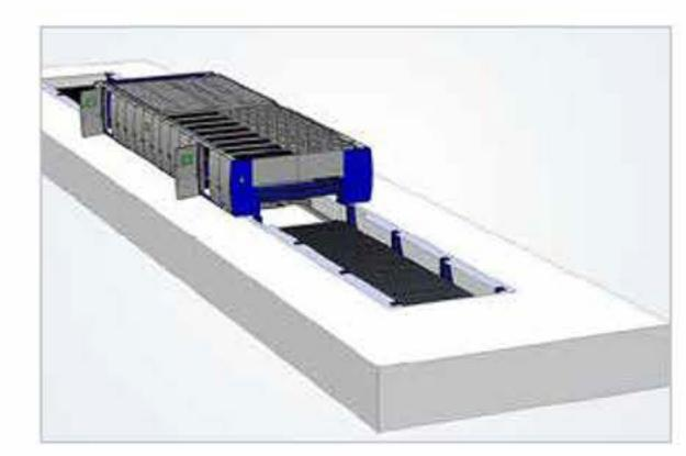
To fit seamlessly into any production facility, MSLoop does not have to stand on the floor. The embedded version with tables returning underground brings considerable benefits, especially loading and unloading at the floor level, and a more efficient fume extraction and scrap removal.
