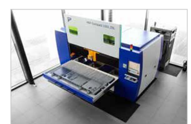
The MSF Compact is available with work areas of 1,000 x 2,000 mm, 1,250 x 2,500 mm and 1,500 x 3,000 mm and is particularly attractive thanks to its small footprint in combination with the genuinely high cutting quality. A manually extractable cutting table enables easy and straightforward loading.
