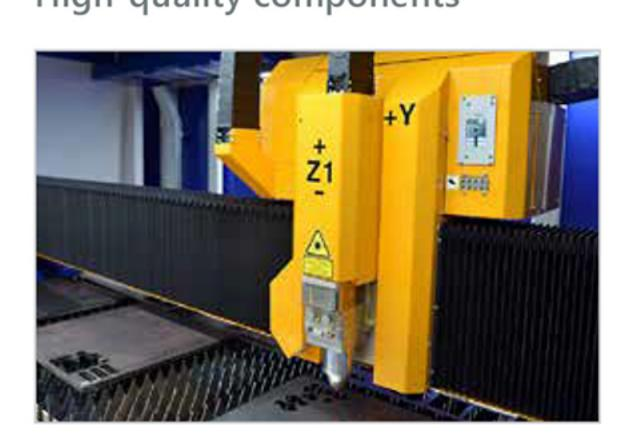
MicroStep relies exclusively on high-quality components from established manufacturers to ensure long-lasting and accurate results. Thus, laser sources from IPG Photonics with a power of up to 4 kW are available. For high cutting speeds, an automatic laser cutting head from the German manufacturer Thermacut is used.
