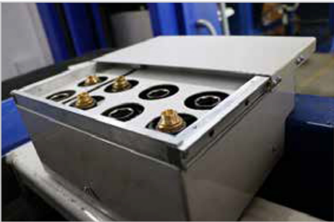
Ever higher efficiency with automatic nozzle changer
