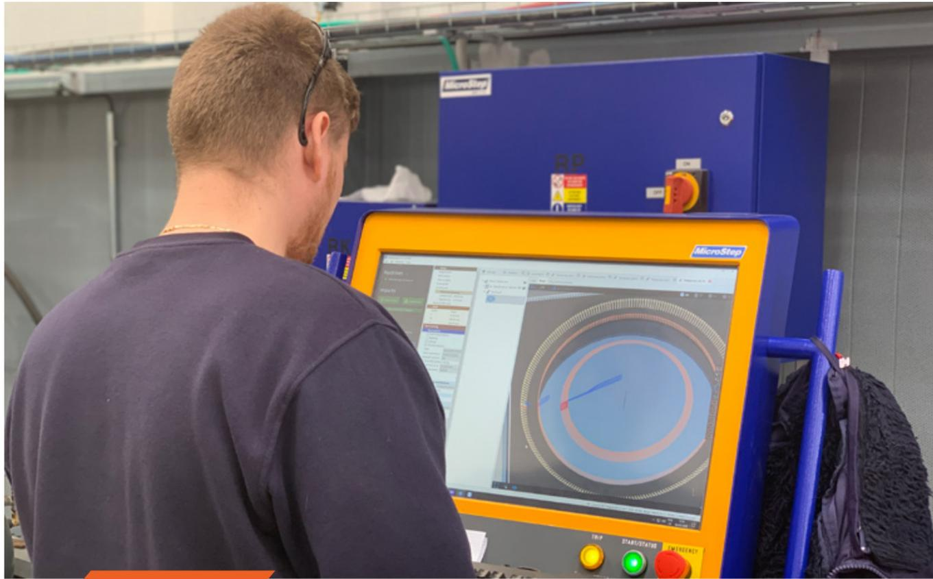
↑ *MicroStep's technology is able to create a detailed 3-D model of an object while fully describing its parameters, including any deviations from the ideal shape.*
