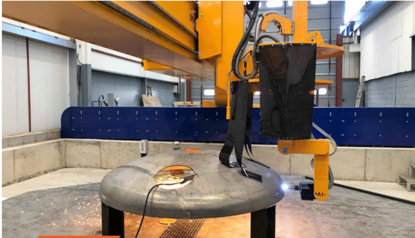
↑ *The software from MicroStep enables a CNC plasma cutting machine to measure the true shape of a 3-D object, such as a dome, and use this information to guide the cutting process.*
