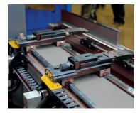
The **large space** facilitates versatile production of parts requiring increased clearance. Ram housing is outside of the machine frame leaving the space between columns free.
