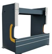
Press brakes feature a **rigid mono-block machine frame** for minimum deflection under load. The steel frame is checked by ultrasound and is stressrelieved after welding. All reference surfaces and connection holes are machined.
