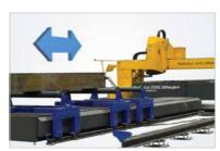
Thanks to the large, open loading area, even heavy beams can be easily and safely slid over the supporting rollers into the work zone. This saves time as the beams do not have to be clamped or otherwise prepared for processing.
