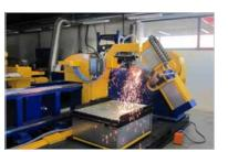
ElbowCut, a special version of the PipeCut machine, was designed for trimming of pipe elbows with preparation of trimmed edges for subsequent welding. The machine can process elbows in the range Ø 80 - 400 mm while ensuring high environmental safety and suction efficiency thanks to housing in a noise reducing cabin\*.
