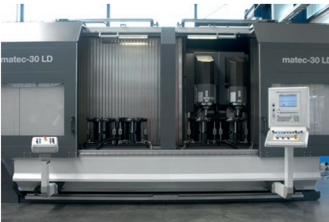
Double spindle: manufacturing of truck wheel hubs
