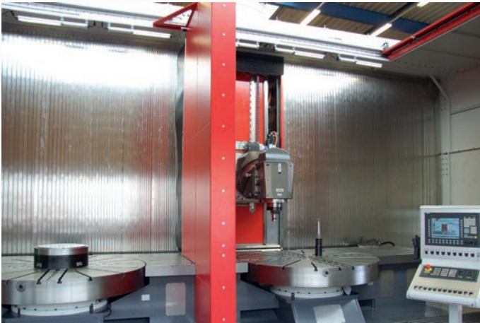
5-sided machining on the rotary table with workpieces up to 2,300 mm length by pendulum machining
