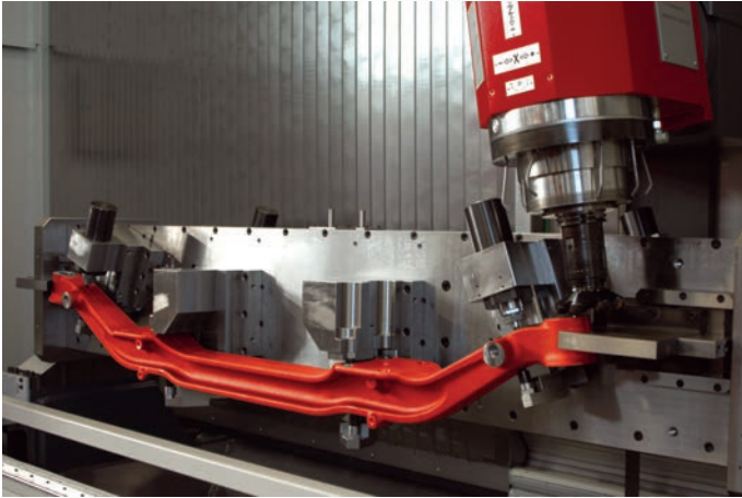
Multi-functional clamping devices on CNC rotary table and counter bearing. Multi-side machining in one clamping position.
