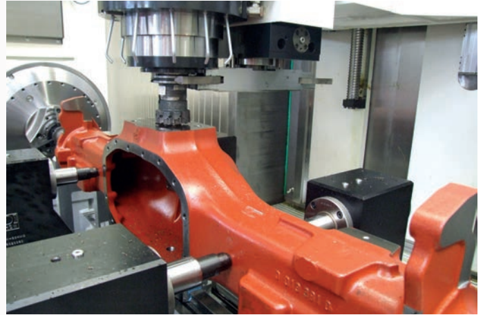
Multi-functional clamping devices on CNC rotary table and counter bearing. Multi-side machining in one clamping position.
