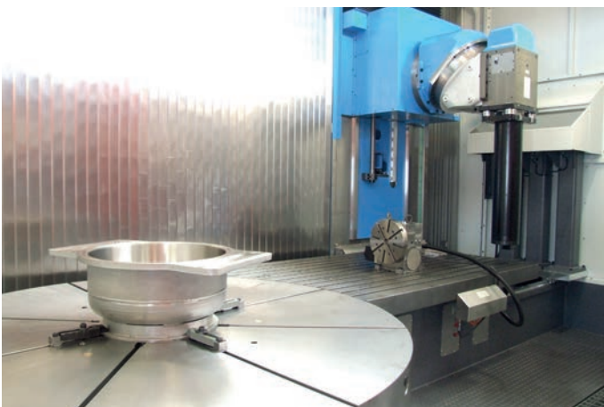
Variant with large rotary table and pick-up milling spindle to dive into large housings
