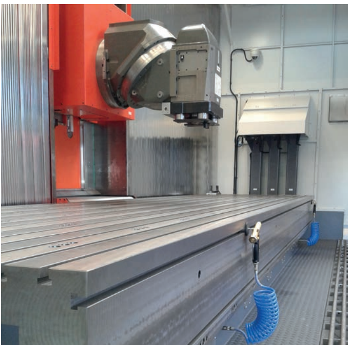
Tool and Mould Making: Machine table with additional vertical clamping surface
