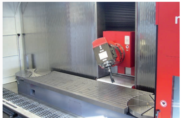
Turn/Mill Center with two rotary tables in pendulum process
