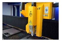
MicroStep relies exclusively on high-quality components from established manufacturers to ensure long-lasting and accurate results. Thus, laser sources from IPG Photonics with a power of up to 4 kW are available. For high cutting speeds, an automatic laser cutting head from the German manufacturer Thermacut is used.
