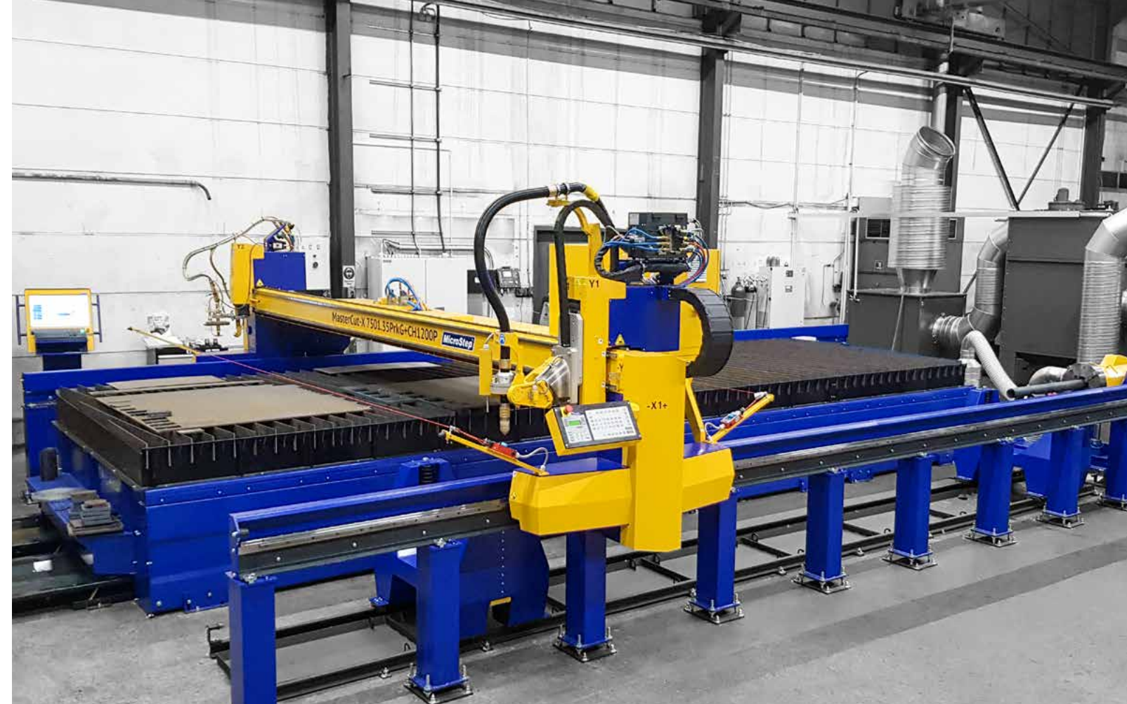
MasterCut with linear guidelines in the X-axis and a channel for pipe processing
