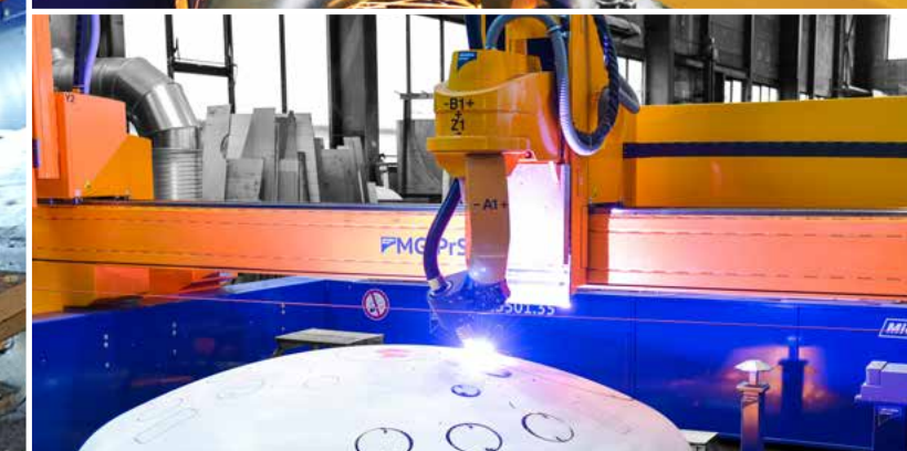
Dome processing with a multi-functional MG cutting machine
