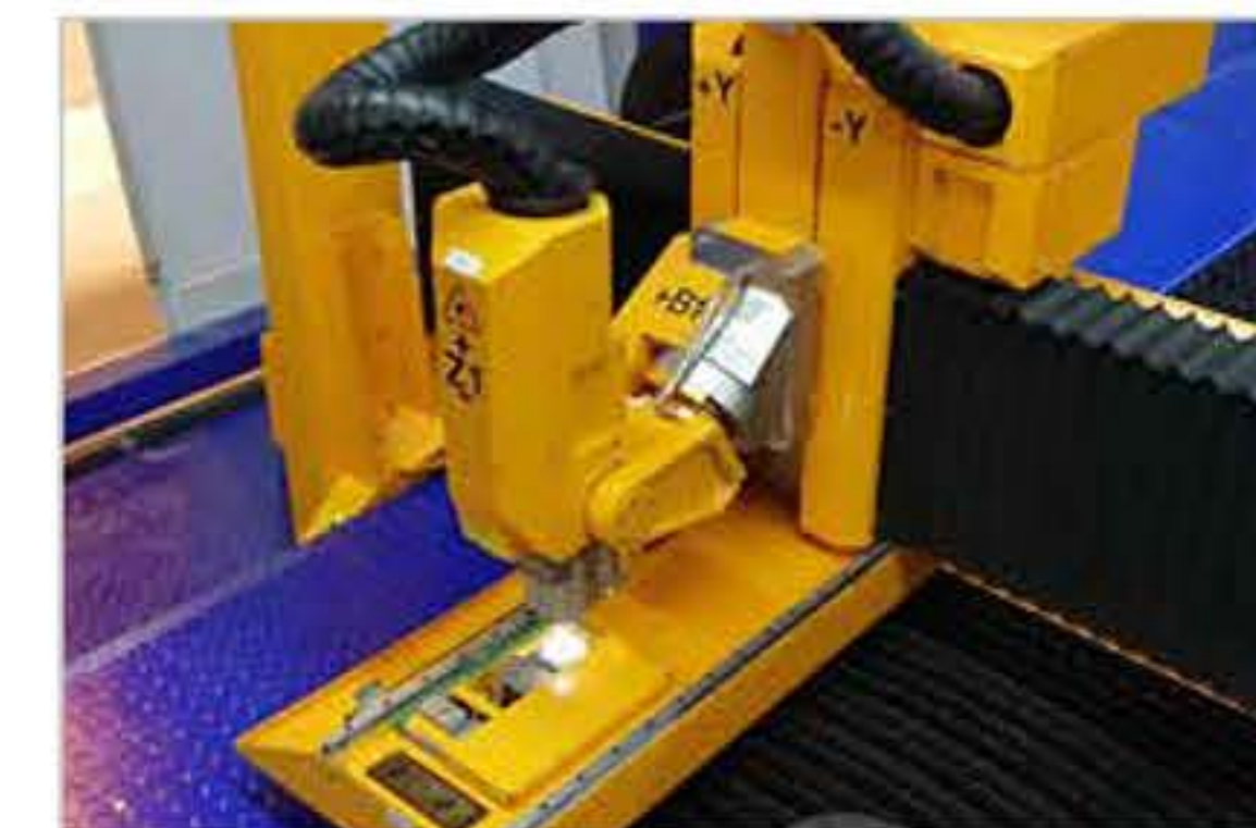
Calibration station with ACTG® unit integrated into the gantry
