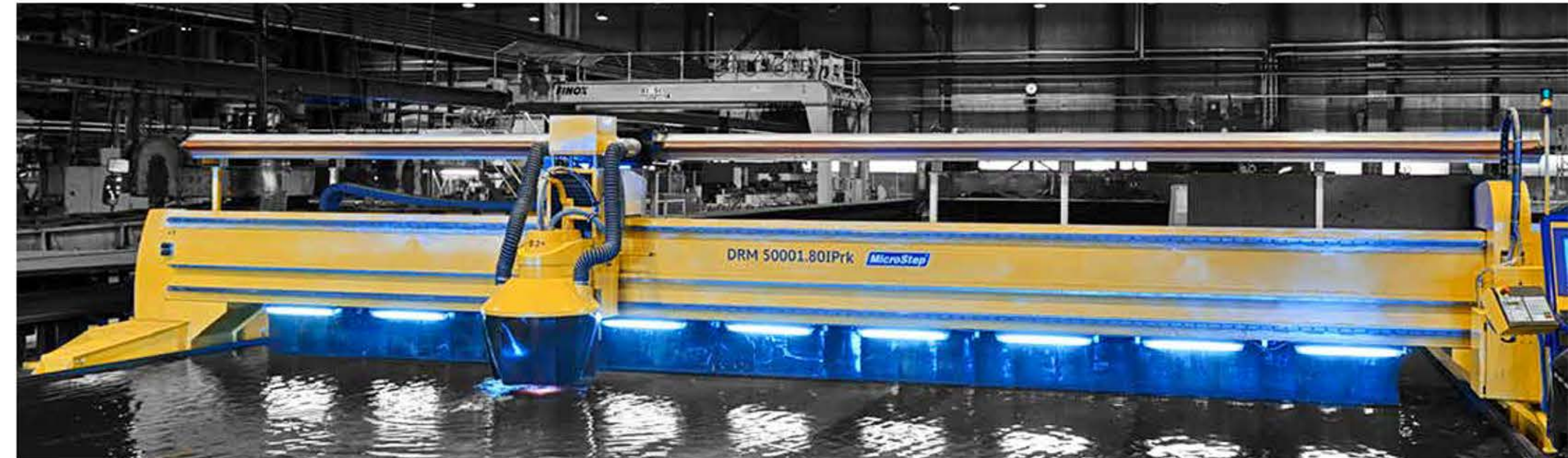
DRM machine with work area 50 x 8 meters and a water table for underwater plasma cutting
