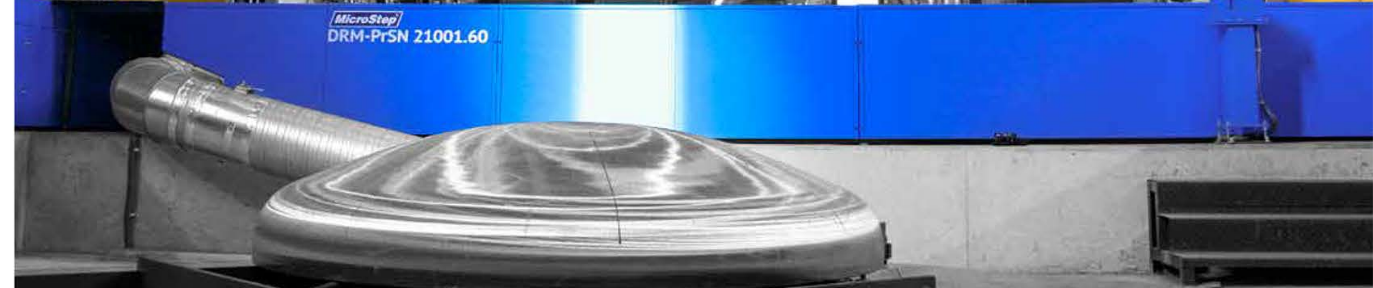
DRM machine for cutting of tank ends up to Ø 5,500 mm
