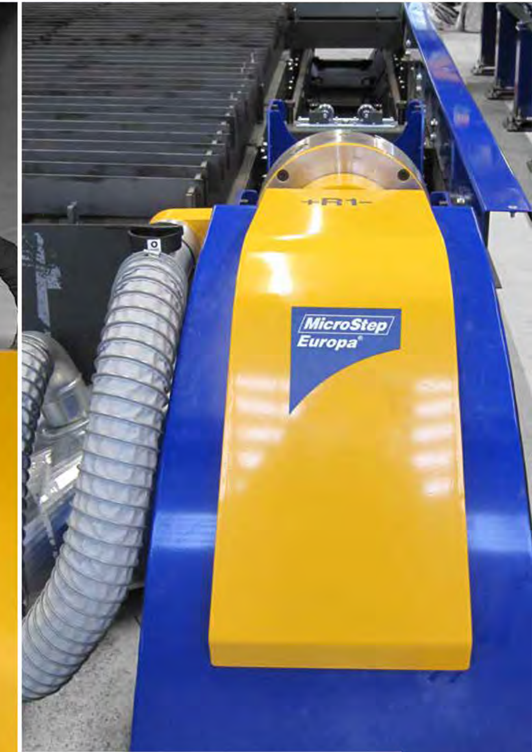
This pipe cutting device can process pipes up to Ø 300 mm
