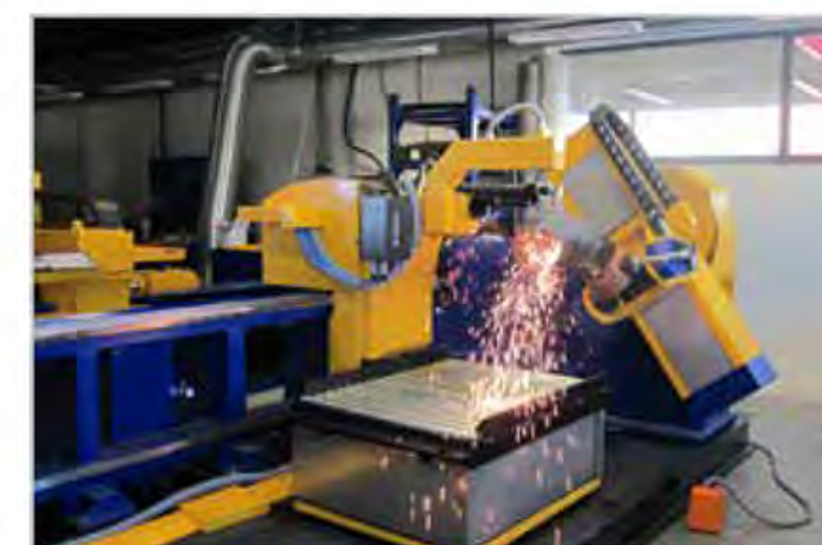
ElbowCut: Weld edge preparation on pipe elbows
