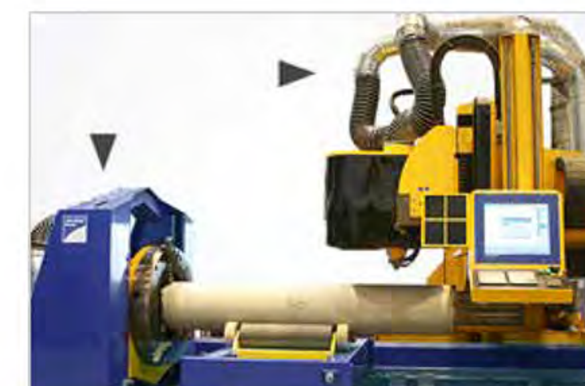
Powerful suction through chuck and the overhead extraction system
