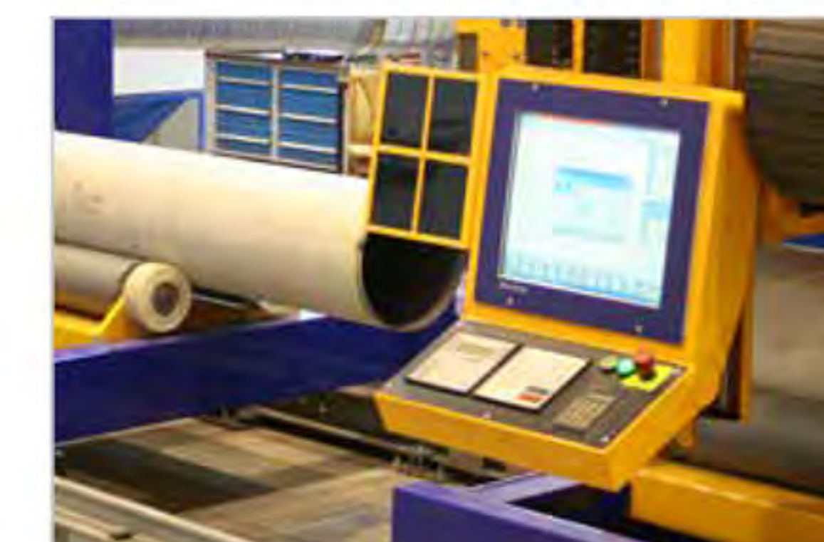
Operator terminal on the gantry
