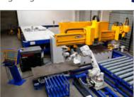
As a time- and cost-efficient production solution, the DS series has a high degree of automation. Loading of plates into the cutting zone, unloading of processed parts as well as separation of residual material are fully automated. The modular design of the machine allows to customize the unloading process incl. sorting by robots. Moreover, the machine is operated by MicroStep's production management software CyberFab® Manager that can be interconnected with local ERP system.
