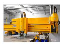
The DS series offers a variety of automated processing options for flat materials. Besides drilling, straight cutting and bevel cutting for weld edge preparation up to  $50^\circ$ , oxyfuel cutting, tapping, countersinking as well as scanning and marking are possible. The standard work area size is up to  $6,000 \times 2,000$  mm.
