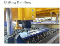
The powerful spindle enables drilling up to Ø 70 mm and a variety of milling operations such as large hole milling, face milling, pocket & slot milling, chamfer milling, thread milling or counter boring.
