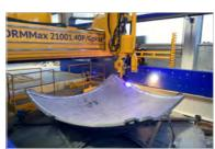
DRM Max can process a whole range of workpieces including domes up to a height of 1,500 mm as well as dome petals. A 3D laser scanner and mScan technology compensate for possible deviations of the real domes for achieving outstanding precision.
