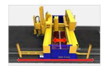
DRM Max gantry features a rigid doublebeam structure with an independent subgantry carrying a 55 kW spindle and two powerful retainers that clamp down with 24,000 N each, over a 750 mm wide drilling and milling area.
