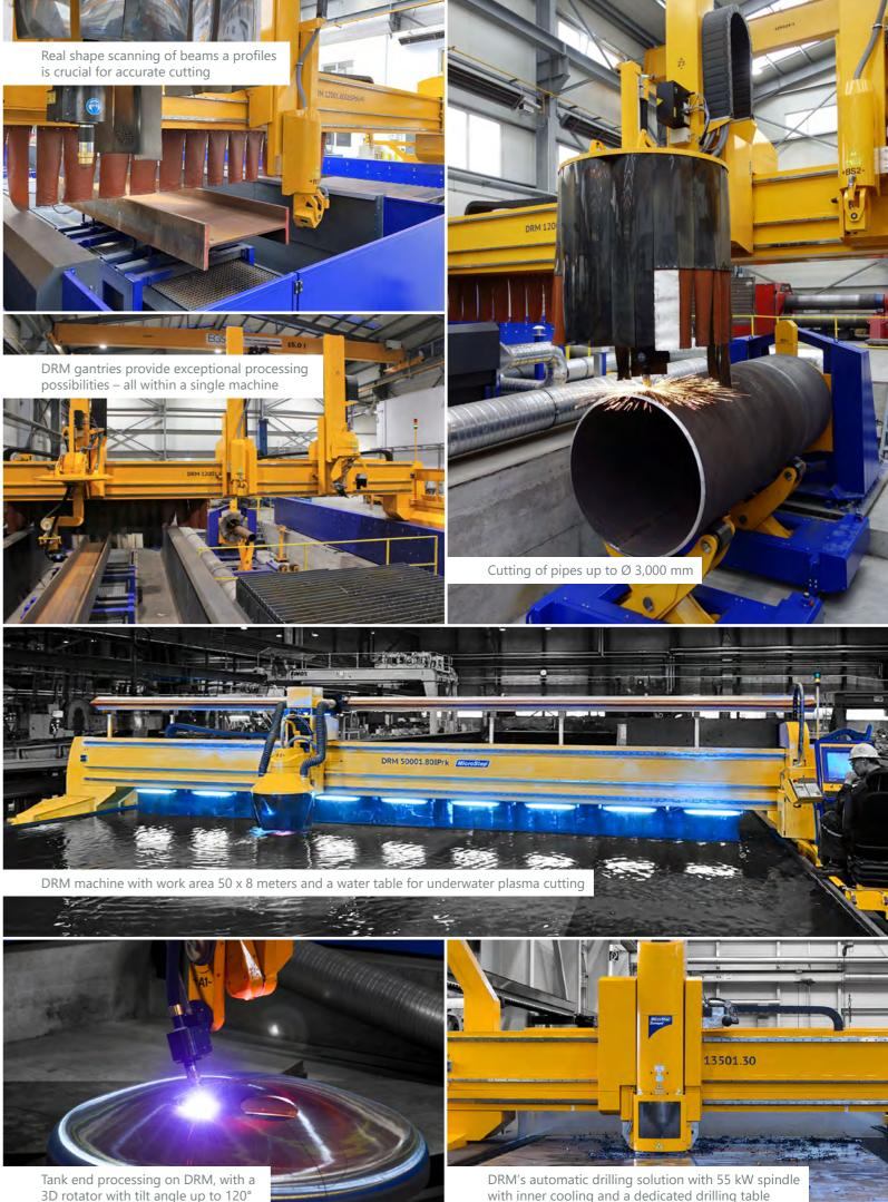
3D rotator with tilt angle up to 120°
